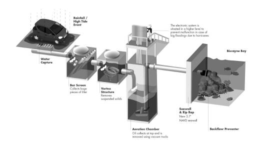
Each of these four steps requires an amount of time to accomplish, so no matter how a system is designed, draining an area of land can never be instantaneous. Each of these four steps offers an opportunity for a bottleneck to develop and slow down the whole process. If the rain falls at a faster rate than any one of the steps can accommodate, the system will back up and ponding (standing water) will occur.
