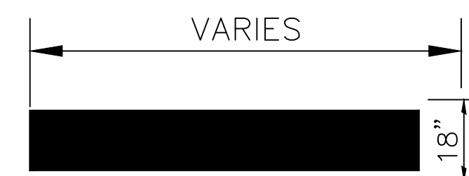
18" SINGLE SOLID WHITE/YELLOW LINE DETAIL NTS NOTE: SINGLE SOLID LINE TO BE THERMOPLASTIC
